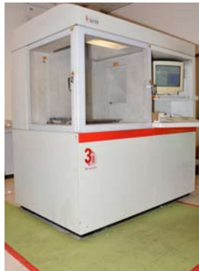
SLA 7000: Components produced by this machine are normally for die and mold inserts, jigs & fixtures. They are suitable for high temperature environments
