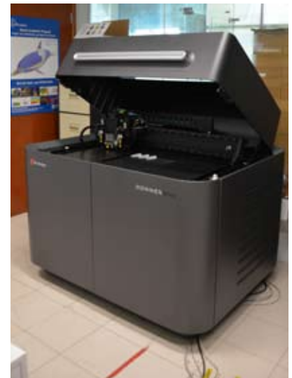
Connex 350: The machine is capable of producing functional prototypes. Common application areas are die and mold inserts and over-mold prototypes
