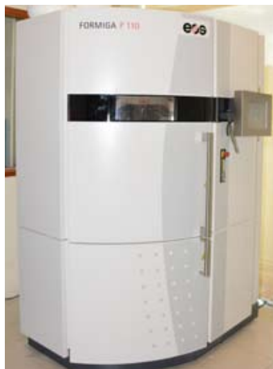
SLS P110: The machine is capable of producing functional prototypes. Suitable for tough and high temperature resistant components
