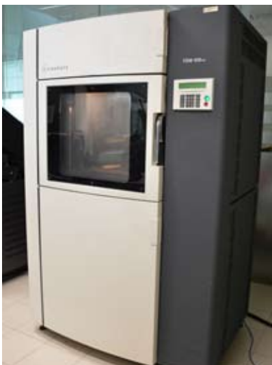
FDM 400MC: Components produced are for form & fit, product illustration and master pattern
